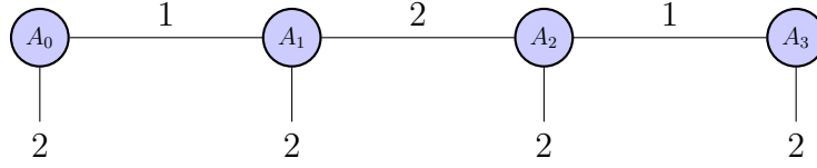
Figure 5.1: A tensor network diagram for binary tensors of order 4 and TT rank (1, 2, 1) .
